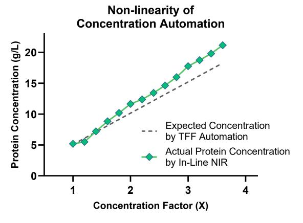
(Left) Expected vs measured protein concentration during the first concentration step. This data indicated that onboard software used by the TFF system did not account for higher or variable protein permeation rates, that were incongruent with scale readings due to changing density of the product. This led to an overconcentration in the initial step, and thus a higher concentration in the diafiltration step, which impacted excipient permeation rates.
