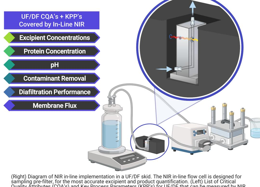
(Right) Diagram of NIR in-line implementation in a UF/DF skid. The NIR in-line flow cell is designed for sampling pre-filter, for the most accurate excipient and product quantification. (Left) List of Critical Quality Attributes (CQA's) and Key Process Parameters (KPP's) for UF/DF that can be measured by NIR. Highlight regions shows principle of measurement for the NIR flow cell design
