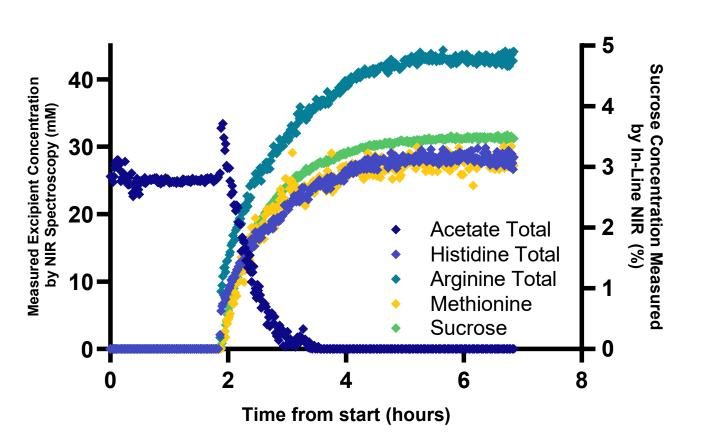
(Left) Real time measurements of all excipients during the first concentration step and the diafiltration step. Diafiltration was performed for the standard 8x diavolume length, by the end of which all monitored excipients were fully exchanged and had reached stable
