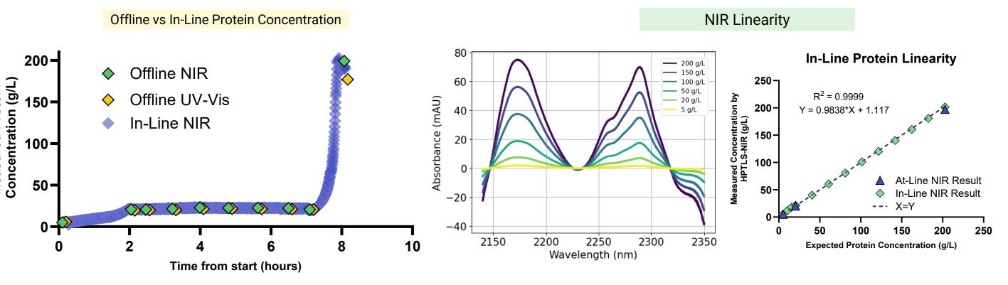
(Left) Comparison of in-line NIR, offline (at-line) NIR, and offline UV-Vis results for protein concentration during the full UF/DF run. Results show good alignment between UV-Vis and NIR, at all stages.
