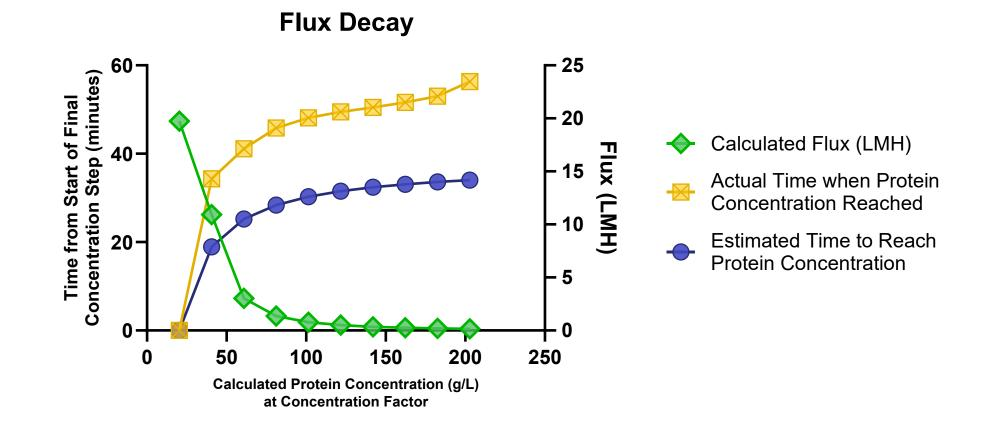
(Right) Real time permeate flux rate, as determined by rate of change of protein concentration as measured by the in-line NIR system. This showed a viscosity or protein concentration impact on permeation – the effect is most notable at concentrations above 50g/L.
