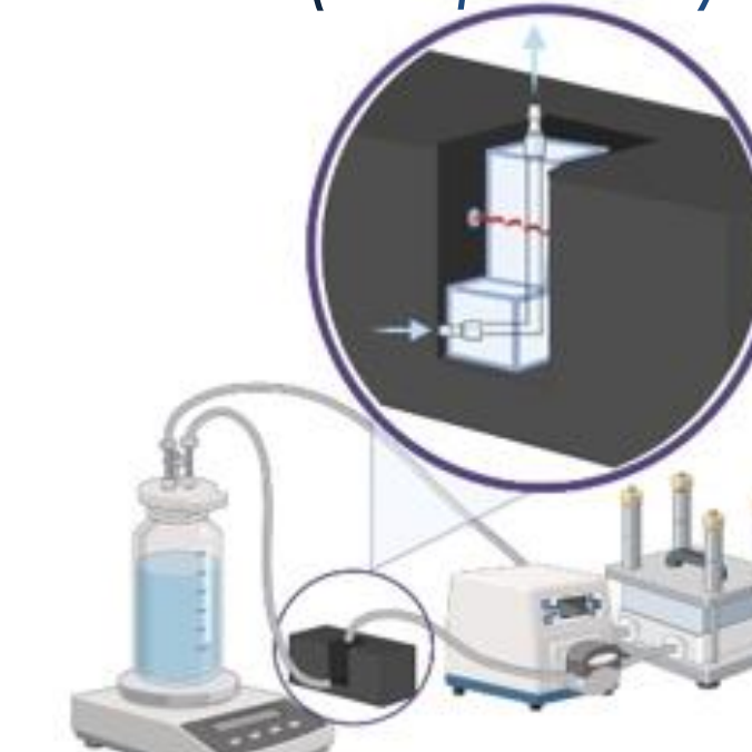
Figure 2: A TFF setup. Highlighted is the removable flow cell in the retentate line and laser path through the sample via optical windows on the flow cell
